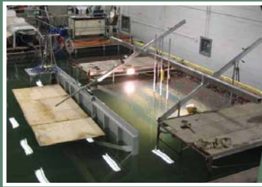
Model Set-Up With The Dike Slope On The Right And Vessel Hull On The Left
